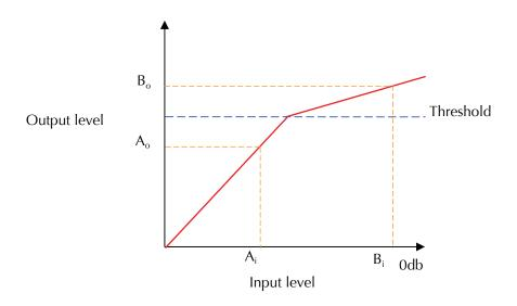
Refer to the diagram above; the red line shows what happens to the signal level when it is passed through a compressor. As you can see when it hits the threshold, the output no longer equals the input; it is lower.
